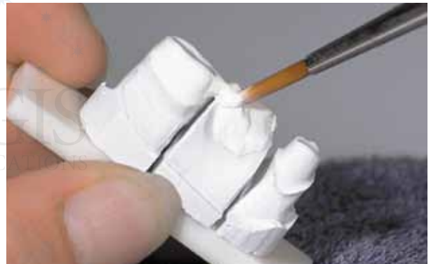
Figure 15 Slip casting an In-Ceram framework.
