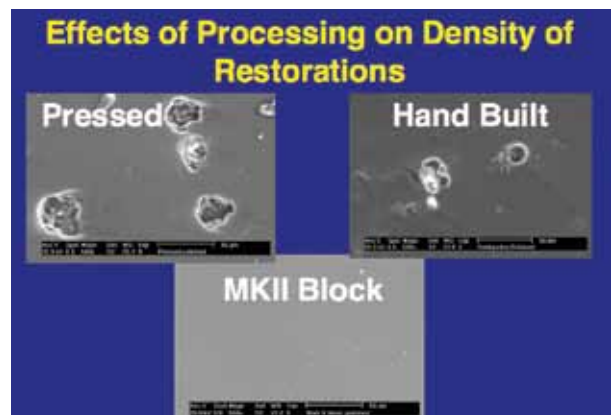
Figure 16 Electron micrograph of the microstructure of a hand-layered porcelain, a pressed crown, and a Vitabloc Mark II CAD/CAM block.
