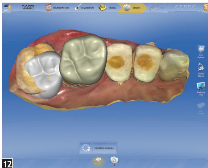
FIGURE 12: After setting the insertion axis, the next step is for the software to calculate the proposal. With the CEREC 4.0 software, anytime a user is treating adjacent restorations, it's recommended for the best results that both restorations be proposed simultaneously. To accomplish this, the margin must be drawn and insertion axis must be set for both restorations prior to proceeding.
