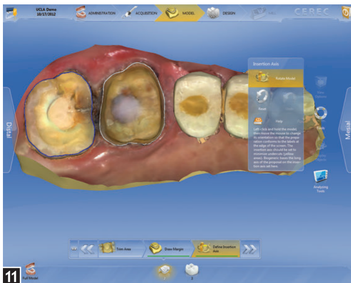
FIGURE 11: Once the first tooth has been margined, the same process is completed with tooth #15. After setting both margins, the Insertion Axis for each case is determined. To set the Insertion Axis, use the visual cues on the right and left side of the screen, and adjust the model accordingly to line up the mesial and distal of the model with the visual cues.
