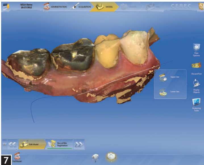
FIGURE 7: The same Edit tool was used to remove bits of the buccal vestibule on the lower jaw. You can see how accurately the Omnicam scanned the natural teeth as well as the existing gold crowns on the patient.
