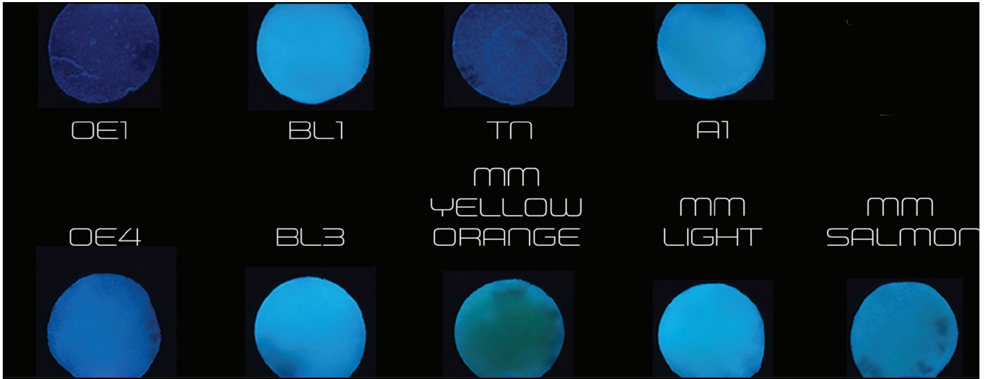
Figure 15: A sample of IPS e.max Ceram powders, all of which demonstrate fluorescence.
