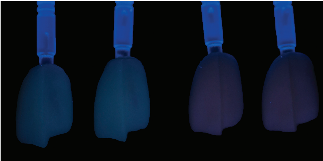
Figure 7: The two crowns (#1 and #2) pressed with the HT A2 ingots appear on the left, while the two crowns (#3 and #4) pressed with the MO2 ingot appear on the right.
