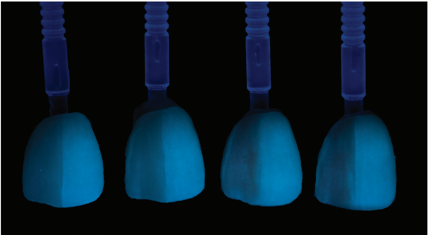
Figure 14: When Fluor Glaze paste was applied and fired on the full-contour half (i.e., right side) of all crowns, the level of fluorescence did not increase much.
