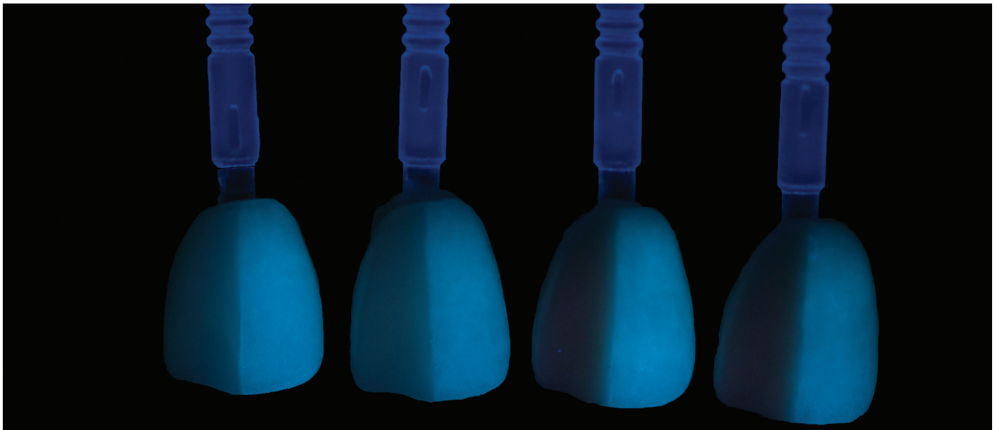
Figure 12: Applying and firing Fluor Glaze paste to crowns #1 (i.e., the HT A2 ingot) and #3 (the MO2 ingot) slightly increased fluorescence.
