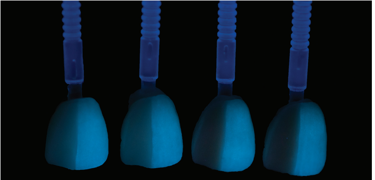
Figure 13: After glazing with Fluor Glaze, the layered half (i.e., left side) of all crowns demonstrated much higher fluorescence than the full pressed half (i.e., right side).
