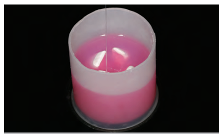
Figure 12 A low-viscosity PVS-duplicating material is poured into the duplicating ring.
