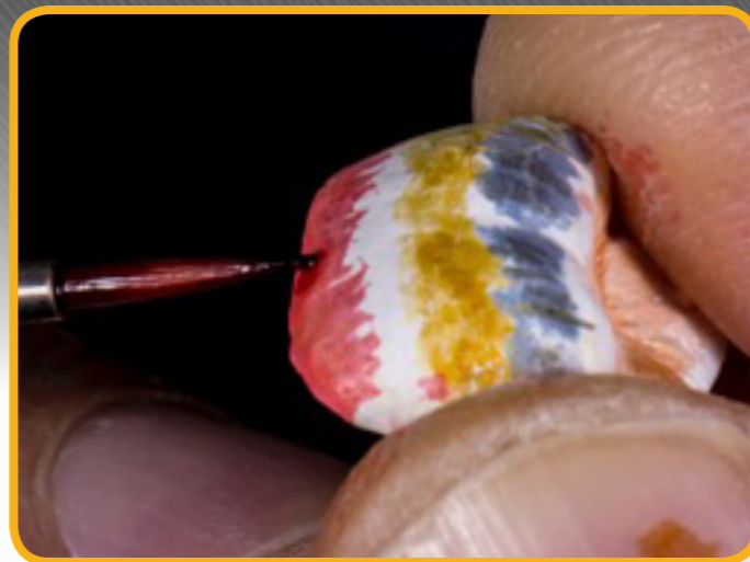
Fig 12. Custom colorizing a CUZR prior to sintering.
