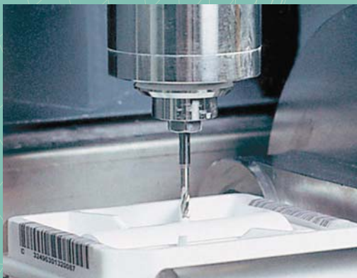
FIGURE 6. A monoblock of zirconia was machined in the laboratory utilizing the Lava system (3M ESPE, St. Paul, MN).
