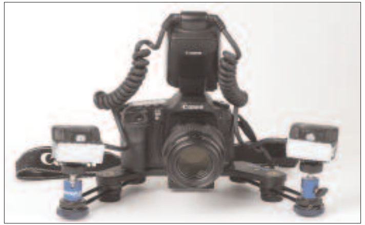
Fig. 7 Canon 20D camera with the Novoflex bracket and the Canon MT 24EX flash.
