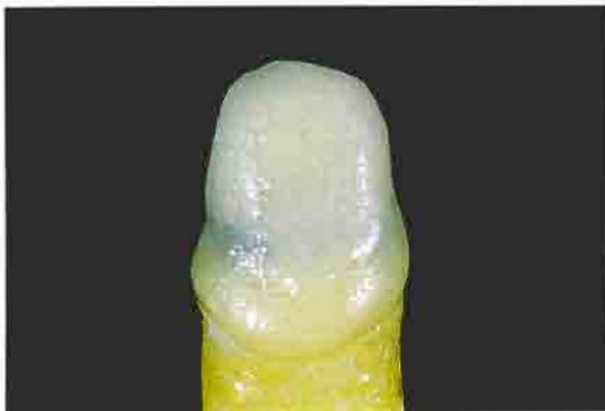
Figure 17A—Vacuum-infiltrated Spinell with Luminaries fired.
