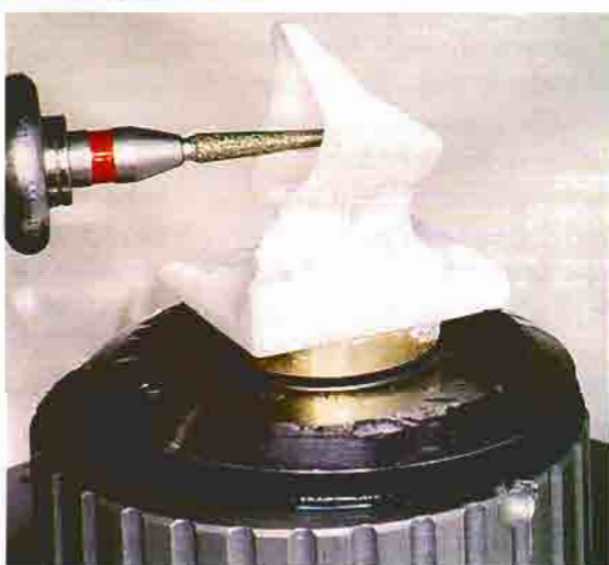
Figure 4 —Milling a coping from a pre-formed monoblock of In-Ceram® Alumina.
