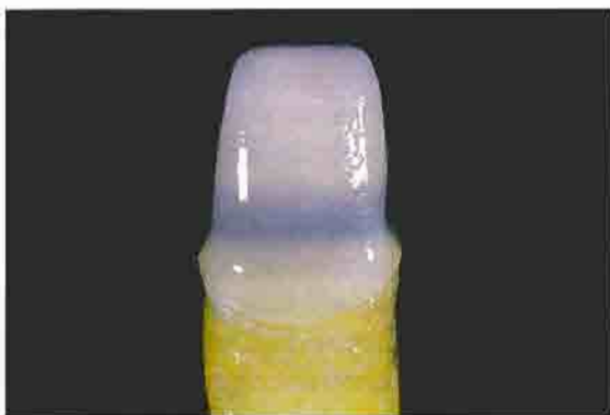
Figure 16C —Spinell coping infiltrated in air. Note the significant increase in opacity.
