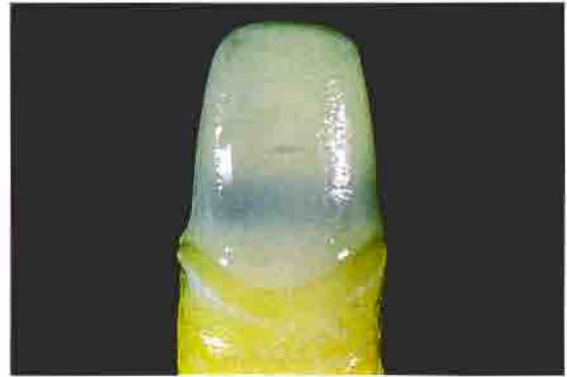
Figure 19B —Vacuum-infiltrated Alumina core demonstrating increased translucency.
