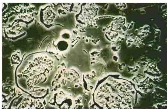
Figure 2 —SEM of conventional ceramics showing the amorphous nature of the glass.
