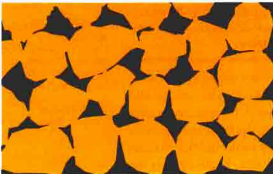
Figure 2 —A schematic of interpenetrating phase materials. There is a partial junction or necking of particles in the crystalline phase. The interstitial spaces between the particles are filled with glass.
