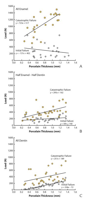
**Figure 3.** Plot of fracture load against porcelain veneer thickness. Initial Hertzian surface cracks are plotted as light blue diamonds, intermediate radial cracks as small black dot, and final catastrophic failures as large blue circles. Regression lines for initial Hertzian surface cracks and final catastrophic failures plotted. A, All-enamel substrate. B, Half-enamel-half-dentin substrate. C, All-dentin substrate.
