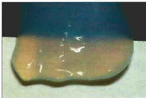
Fig 1 Opal porcelain demonstrating a bluish reflection due to scattering of shorter wavelengths of visible light as the longer wavelengths are transmitted. Once the longer wavelengths (orange/red) hit a reflective surface (as in the white background or dentin), they are reflected back, giving an orange appearance. Some of the orange/red color we see in natural teeth is a result of this effect.
