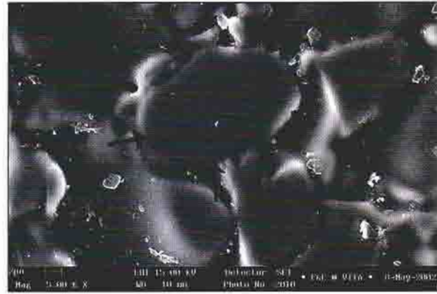
Fig 7 SEM of the previous Alpha material, which has a significantly coarser structure than the new material. This coarseness contributes to its increased abrasiveness relative to finer-structure materials.
