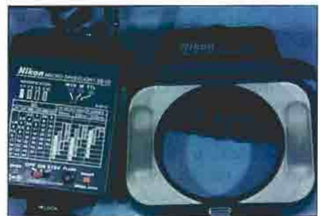
Figure 3. Electronic flash with manual and TTL settings. The flash is set in the TTL mode.
