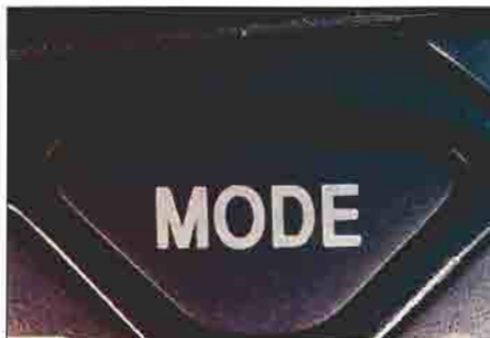
Figures 7a, b, and c. The aperture setting on some cameras will be a simple dial set to A or Ap as in (a); or, in more-sophisticated cameras, an exposure "mode" button (b) is pushed and the dial is adjusted until the LCD screen reads A or Ap (c).
