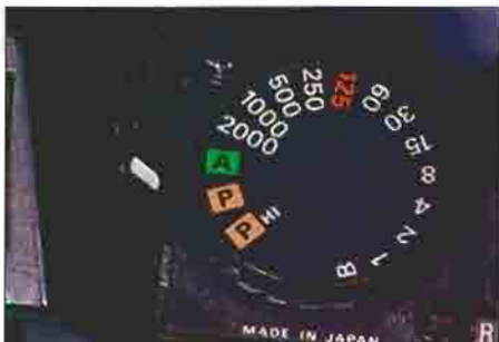
Figures 7a, b, and c. The aperture setting on some cameras will be a simple dial set to A or Ap as in (a); or, in more-sophisticated cameras, an exposure "mode" button (b) is pushed and the dial is adjusted until the LCD screen reads A or Ap (c).
