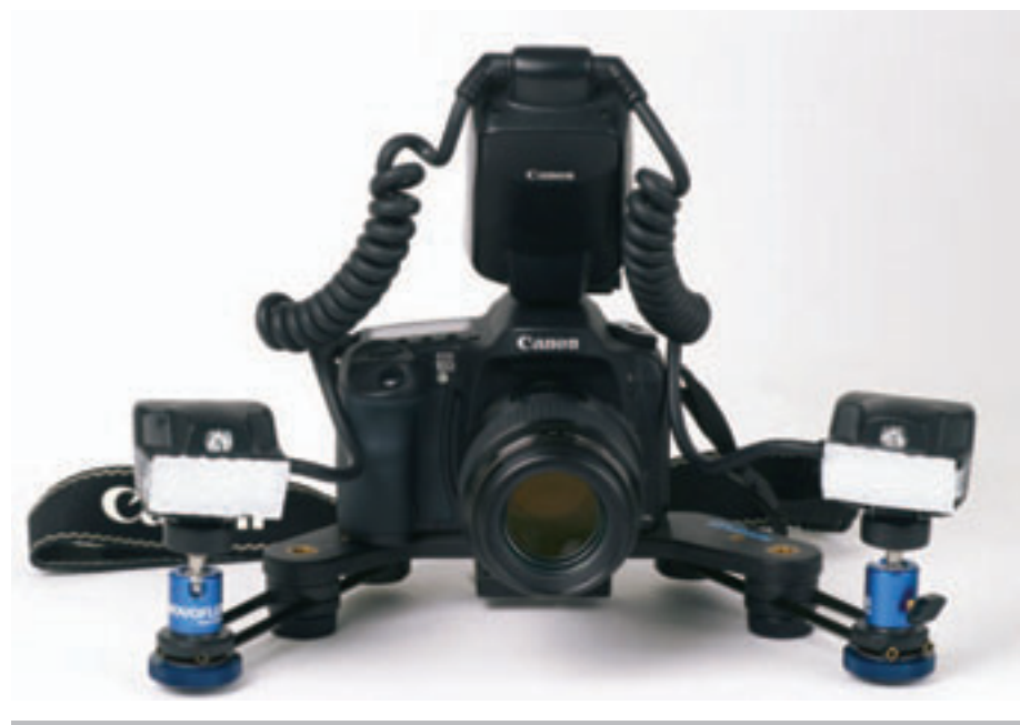
Figure 5 The Canon 20D camera with the Novoflex bracket and the Canon MT 24EX flash.
